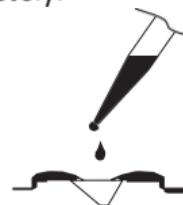
**Note:** If the temperature of the sample differs significantly from the temperature of the instrument, wait approximately 1 minute to allow thermal equilibration.
