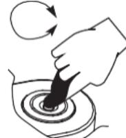
2. Using plastic pipettes, drip sample onto the prism surface. Fill the well completely.
